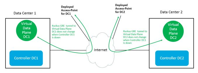
CAVEATS: In this topology, when Data Center 1 is down, Access Point does not have Ruckus GRE Tunnel and WLAN SSID is down. However, the AP SSH tunnel will switch to Controller DC2 and WLAN LBO of AP is still in service.
