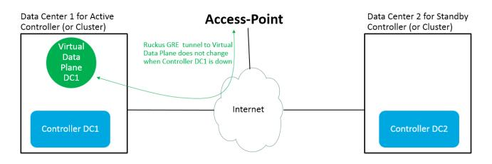
CAVEATS: In this topology, when Data Center 1 is down, Access Point does not have Ruckus GRE Tunnel and WLAN SSID is down
