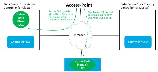
CAVEATS: In this topology, all deployed Access-Point have Ruckus GRE tunnel either with Virtual Data Plane DC1 or Virtual Data Plane @ DC3
