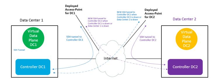
FIGURE 9 SSH Tunnel Between Virtual Data Plane and Controller at each Data Center
